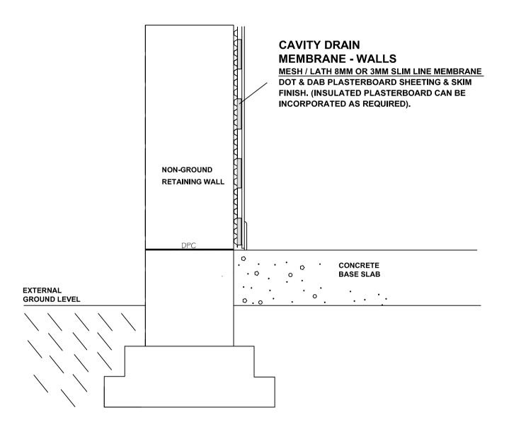
NOTE - THIS DETAIL MUST NOT BE USED ON BELOW GROUND / GROUND RETAINING WALLS
