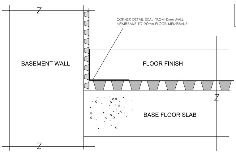
NOTE - THIS SPECIFICATION IS BASED UPON USING THE BLG CENTRAL DRAINAGE SYSTEM BELOW THE FLOOR MEMBRANE. REFER TO ADDITIONAL DRAWINGS FOR FURTHER GUIDANCE.
